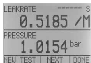
Automatic leak test, adjustable timer and automatic calculation to leak rate / minute
